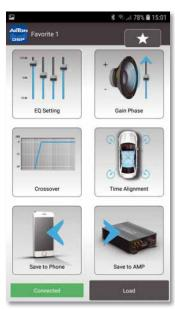
The main menu offers equalization, time alignment, gain and phase, as well as frequency crossovers. The noise gate and the bass-expander are incorporated for gain and EQ
