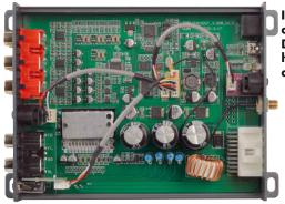
In the A544DSP located at top center are the DSP, controller and the helpers for Bluetooth and digital inputs
