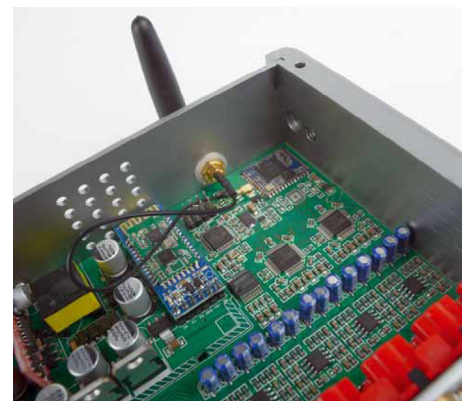
Located in a rear corner are the Bluetooth chips and both DSP cores
