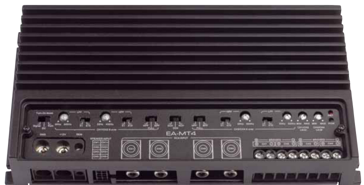
The control panel is concealed under aluminum covers; there are separate high and low inputs
