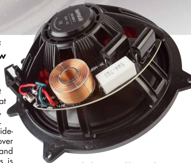
12 dB low pass filter and a bypass sit on the circuit board that is attached directly to the woofer basket
