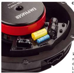
also plug & play connectable. Here too a second-order filter made up of a capacitor and inductor ensures the sound is right. The Emphaser is therefore provided with a quite sophisticated crossover compared to vehicle speakers of simpler construction. The only thing small about the tweeter is the housing: its 28 mm voice coil together with woven fabric dome are rather above the class average.
