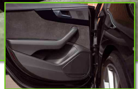
There is space at the rear for a 16-cm two-way system
