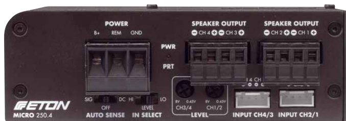
Power and speakers are connected via plugs
