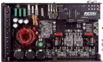
The right half accommodates the amplification section together with the two driver ICs. The power transistors lie under the circuit board
