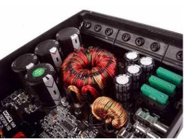
The generously designed power supply unit is good for more than 2 x 400 watts
