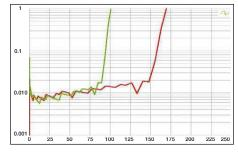
With the Power 150.6 it is simply astounding how it cranks out so much power at such low distortion. Up to 150 watts channel output the distortion remains under 0.02 %
