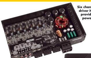
Six channels each with a Class D driver IC and two MOSFETS provide more than impressive power reserves
