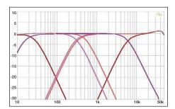
The crossovers of the 150.6 are asymmetrically split over the channel pairs. Channels 5 and 6 are specially for bass, while 1 and 2 can also run tweeters
