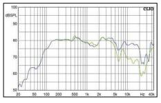
The external crossover separates the RSX 80 as a full-range speaker with super tweeter. The frequency-amplitude response gives no cause for concern.
