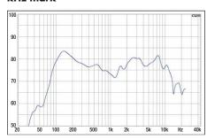
The center speaker covers the frequency range from 100 Hz to 10 kHz, which is all you need
