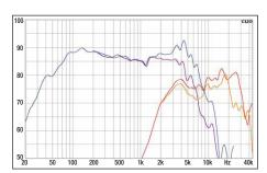
The 16 cm woofer for the doors runs almost like a straight line below the corner. The tweeter operates over of a very wide band to well over the 20 kHz mark
