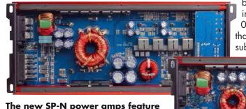
The new SP-N power amps feature a modern class D layout. In the right half the encapsulated lowpass coils can be seen behind the reinforcement
