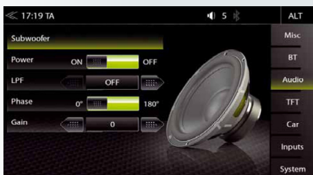
Cut off frequency, phase and gain of subwoofer
