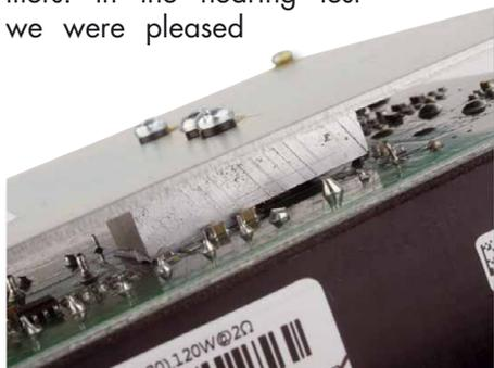
**At the rear of the amplifier module an unassuming aluminum heat sink block indicates that here we are dealing with power electronics**
