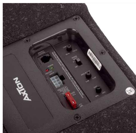
**The small amplifier module has controls for sensitivity, boost, low pass and phase**
