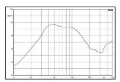
That is textbook bandpass tunina: Superb amplitude response down to almost 30 Hz in the basement with a crisp 88 dB at 1 watt
