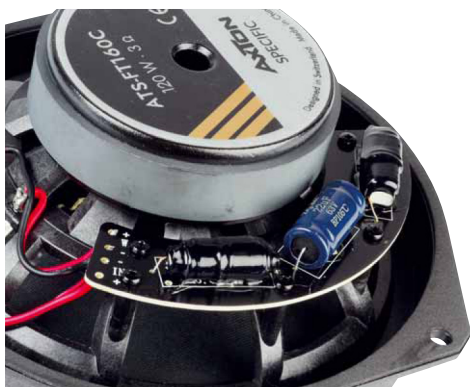
Elaborate crossover with low pass and RCL circuit
