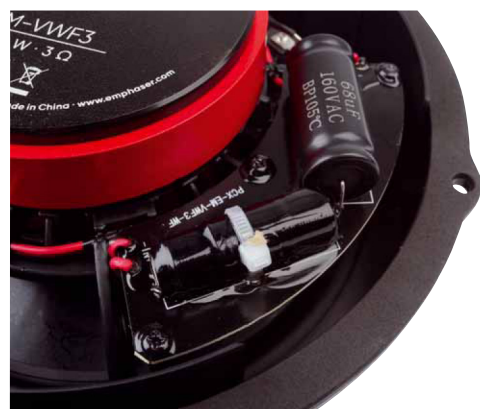
Practical: Woofer branch of crossover on basket with voice coil and capacitor
