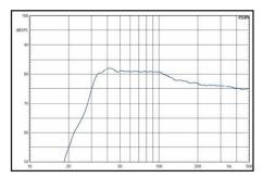
The EBR-M8DX is a good example of a flat and balanced response while still delivering full level in the lows. With 81 dB at one watt it is very quiet, and this will have to be compensated for by amplification
