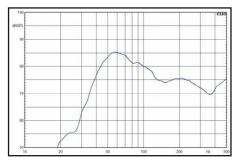
The EBR-M10DX concentrates on its preferred frequencies from 45 Hz to 60 Hz, boasting 85 dB at one watt
