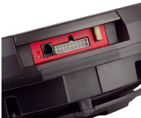
A single Molex connector brings all the wiring together
