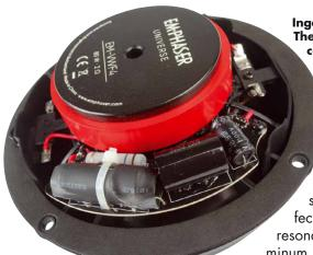
Emphaser offers here for the VWF4 is anything but a cheap solution. A laminated core inductor and an MKT capacitor in this position is a good practical choice; then comes the addition of an RC element for optimization – even external crossovers cannot offer anything better. For the tweeter there is a level resistor and a film capacitor. A vehicle-specific system requires no adjustment controls: due to the fixed mounting positions of the speakers it either fits or it does not
