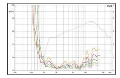
The total harmonic distortion of 96 - 108 dB (0.5 m, with crossover) is wonderfully low, only at extreme levels it rises harmlessly above 10 kHz.
