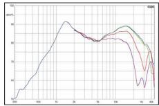
In the baffle and without a crossover, the CXS 28+ bucks in the range of its self-resonance, which has to be ironed out by the crossover. For a 28 millimeter dome tweeter, the Eton loses just little output off-axis.
