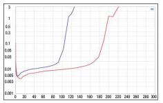
Almost 200 watts into 2 ohms is the maximum channel output. Into 4 ohms it is 113 watts with a very low distortion, which makes the MA 6 among the more powerful multichannel units
