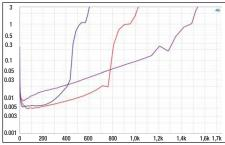
Full-range power at somewhat less than 600, 1000 and 1300 watts with little distortion
