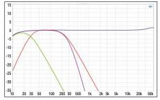
The MA 1 runs full-range and slowly comes to an end only at 50 kHz-not bad at an output of well over 1 kW
