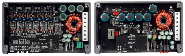
Large sized power supply units, lots of electrolytic capacitor buffers, encapsulated filter coils—the design of the MA amps promises a lot of power just by the appearance
