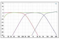
The MA 6 has crossovers for its three channel pairs suitable for filtering everything from subwoofers to tweeters. Here too there is a HiRes capable frequency response up to 50 kHz
