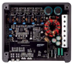
For the MA 4 there is a 4-channel driver chip and the same superb flat wire coils. At the top four pairs of MOSFETs can be seen
