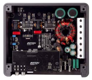
Each channel of the MA 2 has its own driver chip, the power transistors being mounted under the circuit board
