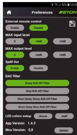
The basic settings (preferences) cover color selection for remote control and amp, converter filter characteristics, and buttons for adjusting the sensitivity of inputs and outputs
