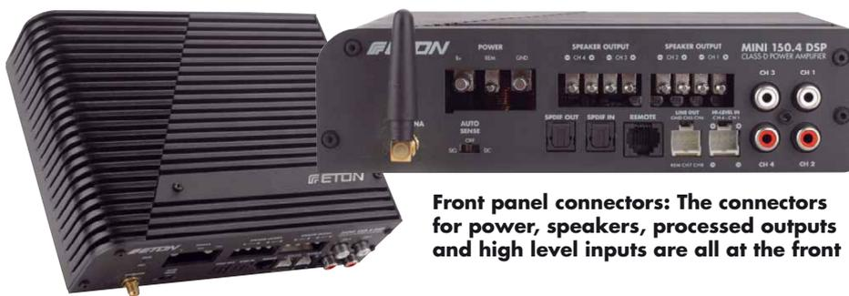
**Front panel connectors: The connectors for power, speakers, processed outputs and high level inputs are all at the front**
