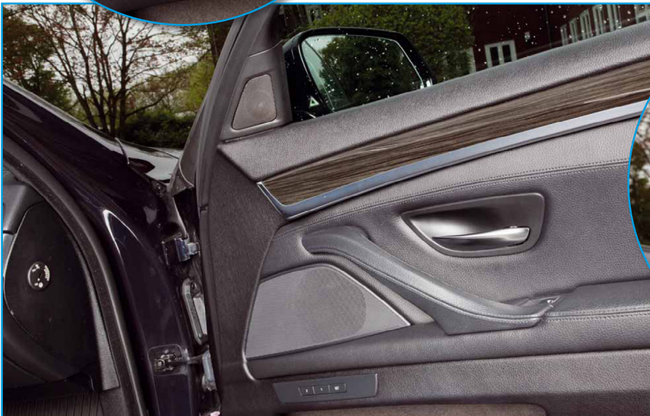
The BMW doors have space for one of the three 10-cm mid-range speakers
