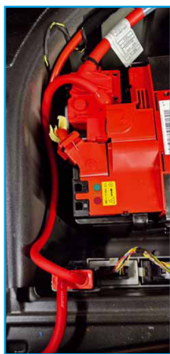
The Eton cable kit with 20 mm² power cable is easily adequate for the installed amplifiers
